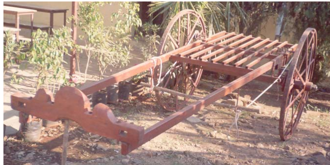
Fig.2: 0.5 Ton Carrying Capacity Bullock Cart
