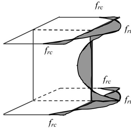
**Fig. 15 Residual stresses in I beams**
