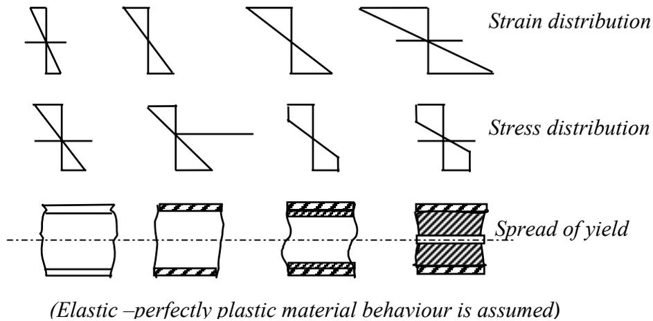
**Fig 13 Strain / Stress Distribution and yielding of section**
