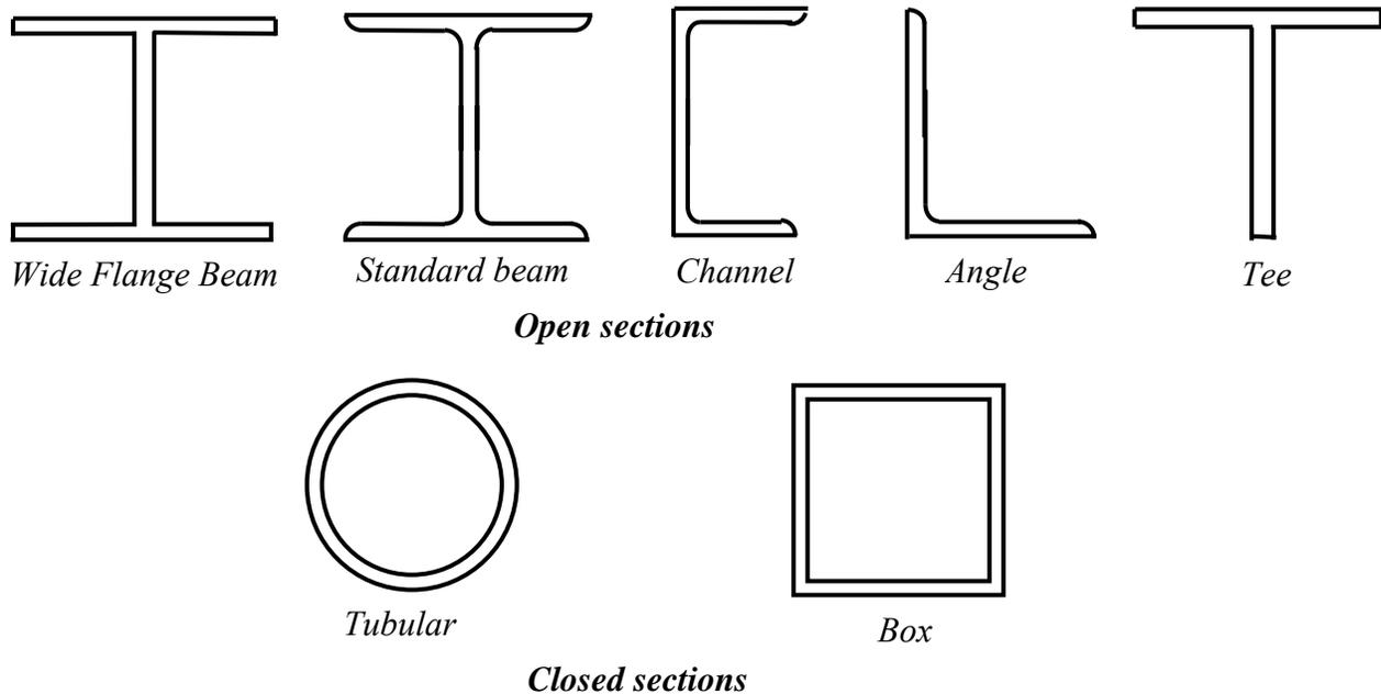
**Fig. 4 Open and closed sections**
