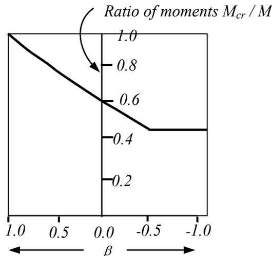
**Fig. 8 ‘m’ factor for equivalent uniform moment**
