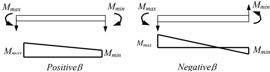
**Fig. 7 Non uniform distribution of bending moment**
