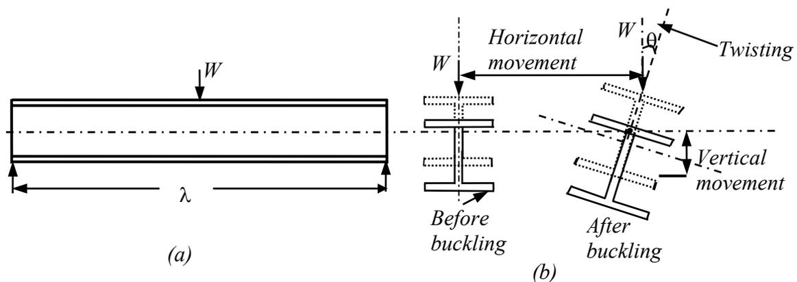
**Fig. 2(a) Long span beam, (b) Laterally deflected shape of the beam**
