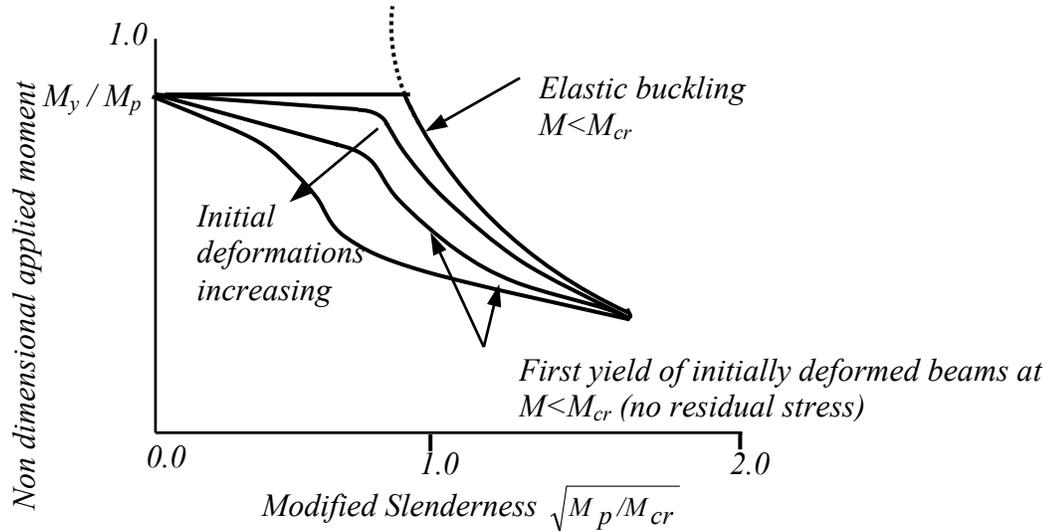
**Fig. 16 Beam failure curve**
