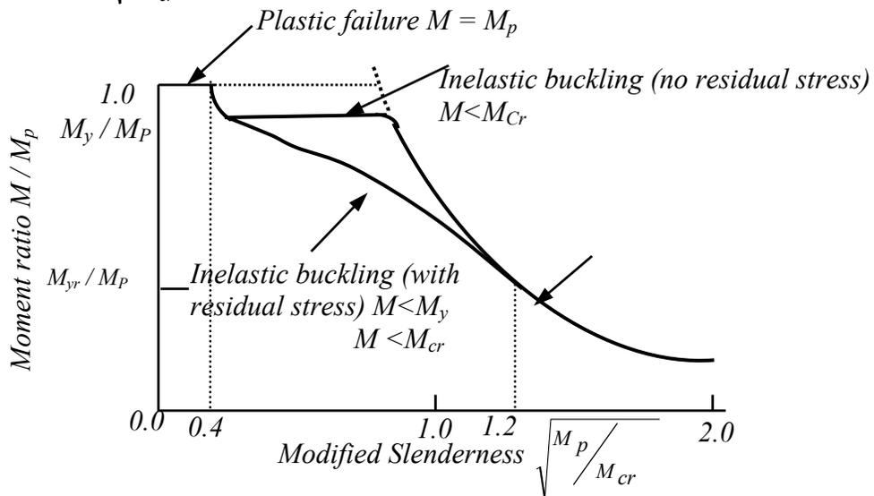
**Fig. 14 Interaction between instability and plasticity**
