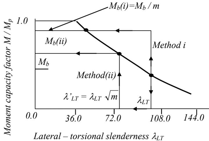
**Fig. 10 Moment capacity of beams**
