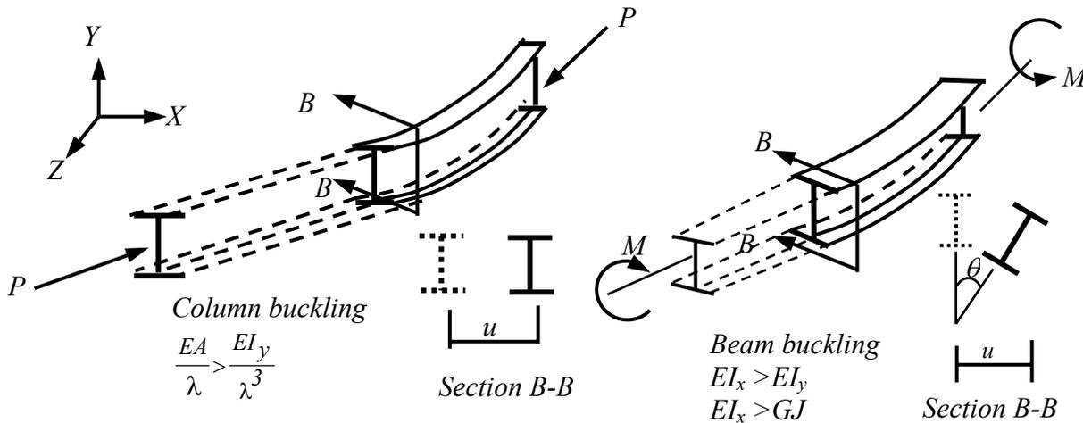
**Fig. 3 Similarity of column buckling and beam buckling**
