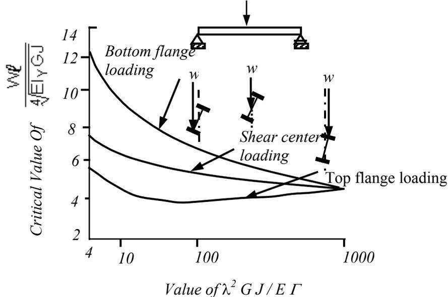
**Fig.6 Effect of level of loading on beam stability**
