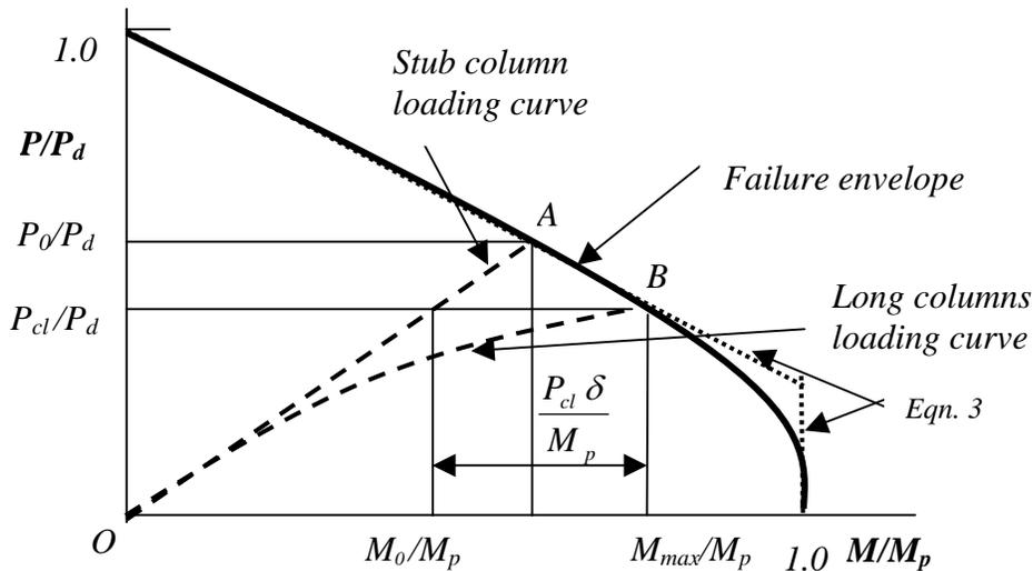
**Fig. 3 Beam-Column Failure Envelope**
