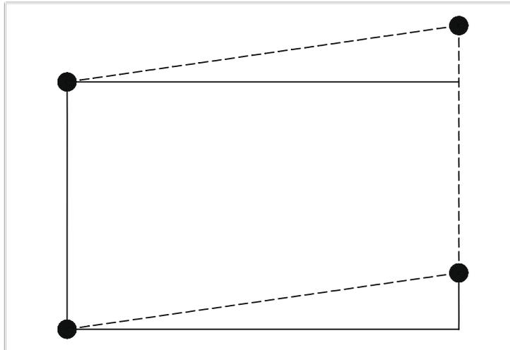
Fig. 8 Picture frame mechanism of strong flange
