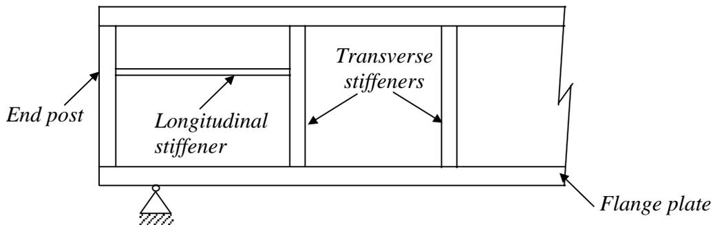
**1.3 Recommended proportion of flanges** *Fig. 2 End panel strengthened by longitudinal stiffener*
