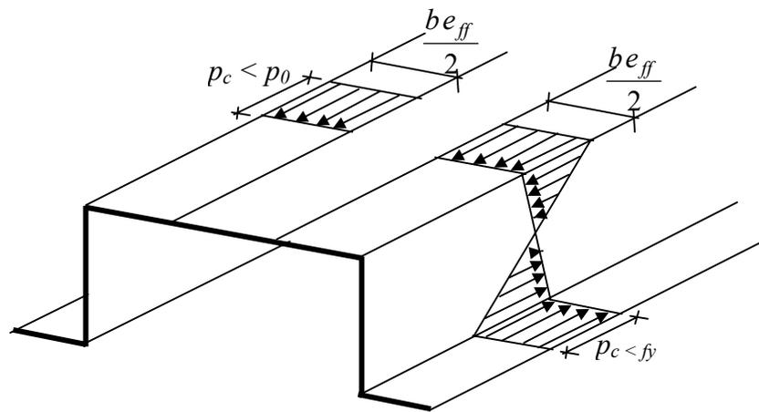
(a) Failure by compression
