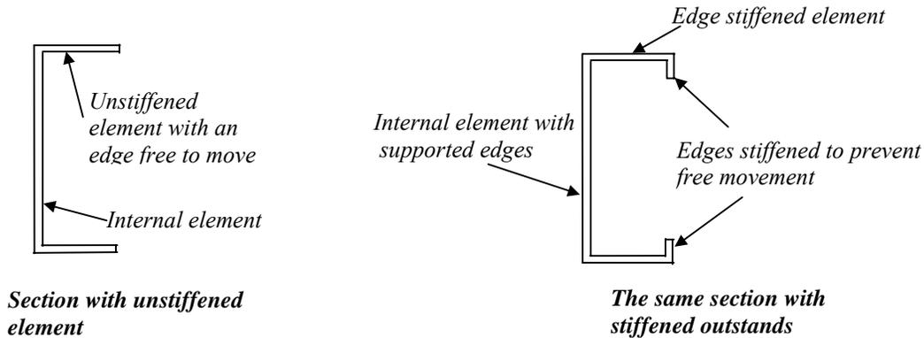
**Fig. 4 The technique of stiffening the element**
