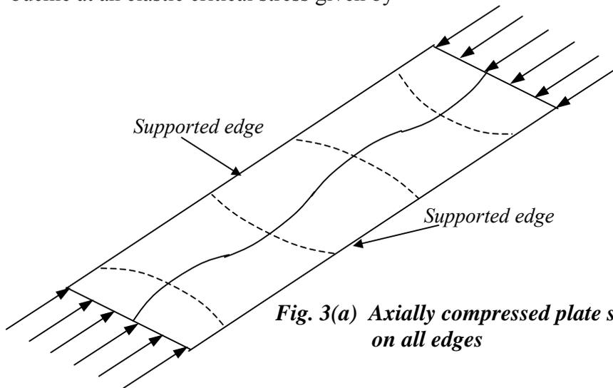
*Fig. 3(a) Axially compressed plate simply supported on all edges*
