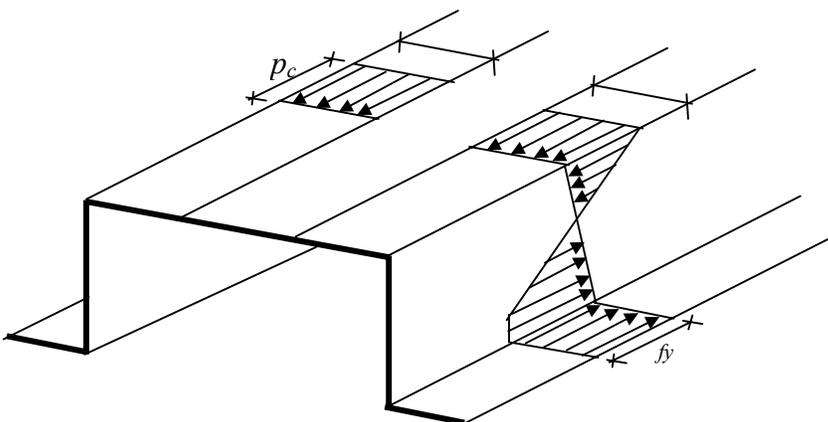
(b) Tensile stresses reach yield before failure-
