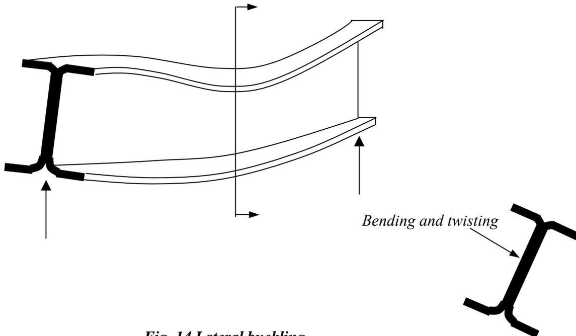
**Fig. 14 Lateral buckling**
