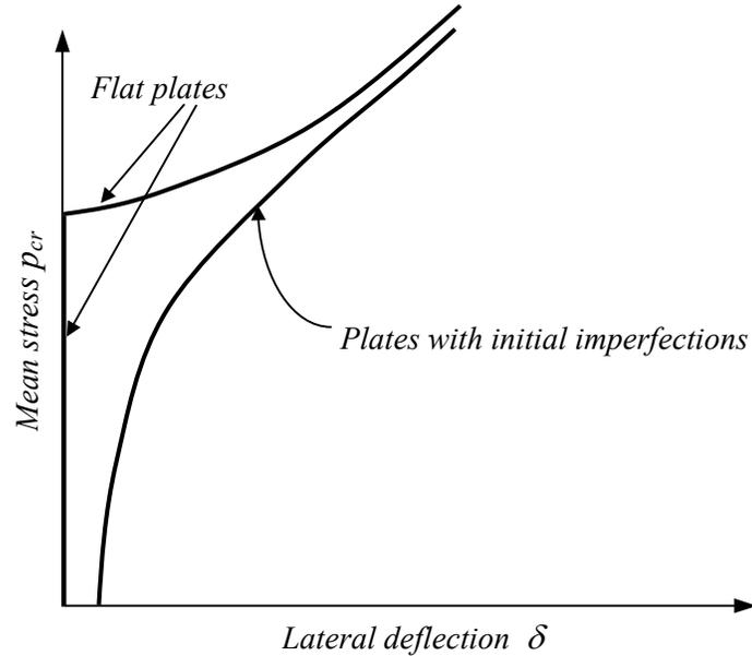
**Fig. 6 Mean stress Vs Lateral deflection relation**
