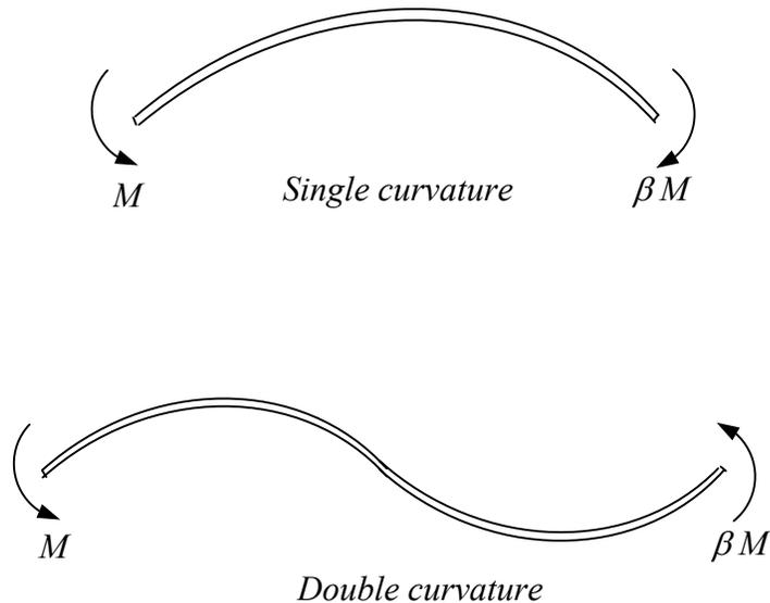
**Fig. 15 Single and double curvature bending**
