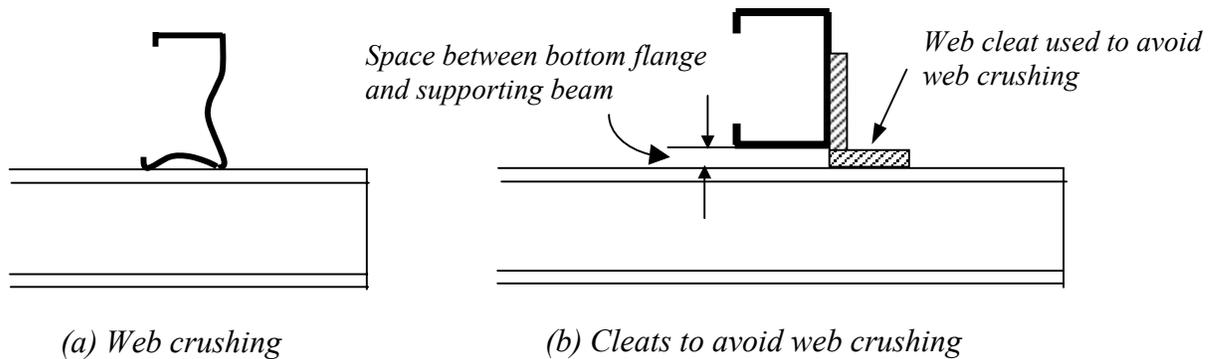
**Fig.12 Web crushing and how to avoid it**
