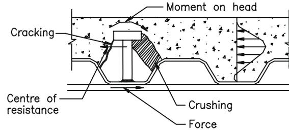
**Fig. 15. Behaviour of a shear connection fixed through profile sheeting**
