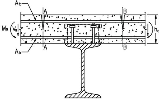
**Fig.17. Surfaces of potential shear failure**
