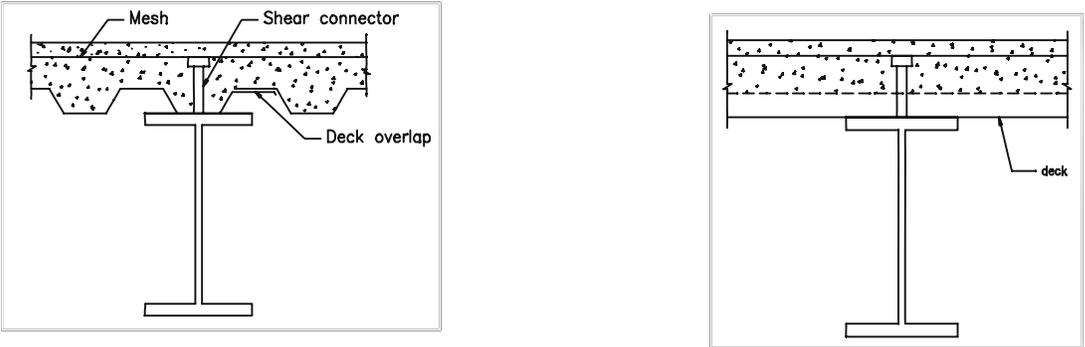
(a) Ribs parallel to the beam (b) Ribs perpendicular to the beam
