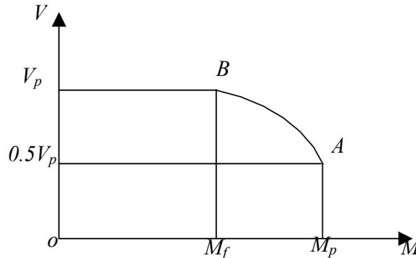
**Fig16 Resistance to combined bending and vertical shear**
