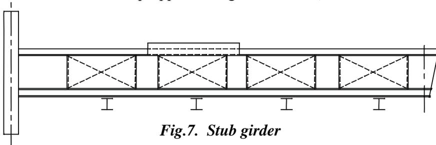
*Fig.7. Stub girder*
