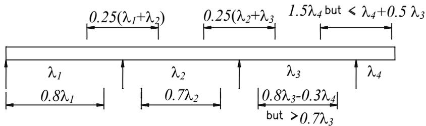
**Fig. 10 Value of  $\lambda_0$  for continuous beam as per EC4**
