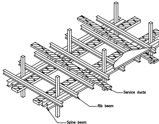
**Fig. 5. Parallel beam grillage**
