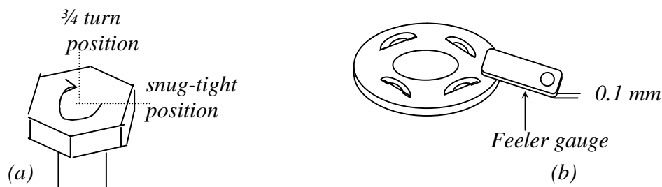
Fig. 5 Tightening of HSFG bolts
