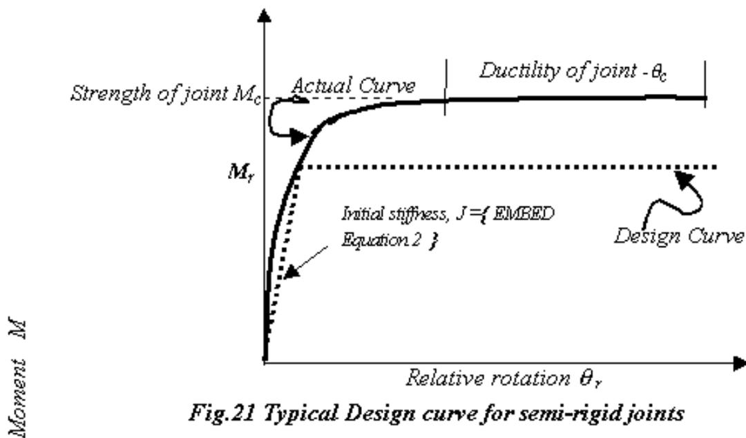
Fig.21 Typical Design curve for semi-rigid joints
