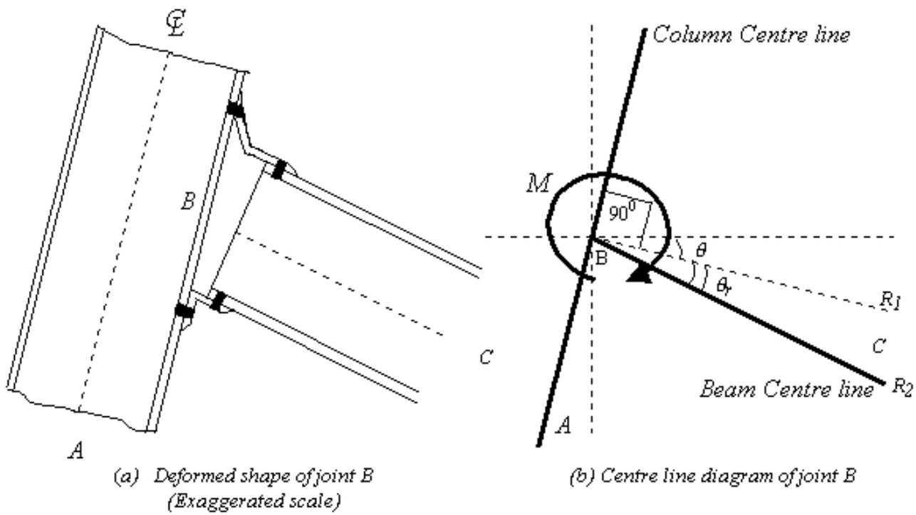
**Fig.2 Connection flexibility of beam-column joint**
