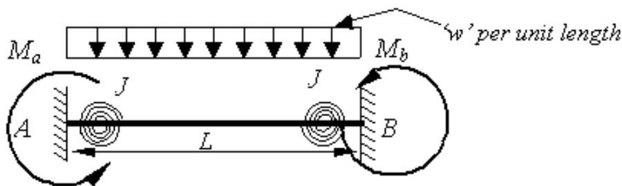
**Fig.11 Beam with UDL and flexible connections at both ends**
