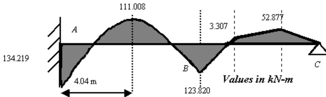
Fig.19 Bending Moment Diagram (flexible case)
