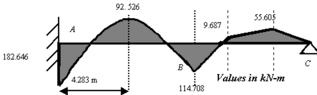
Fig.17 Bending Moment Diagram (rigid case)
