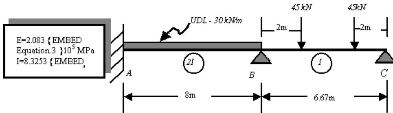
*Fig.16 Continuous beam with rigid connections*
