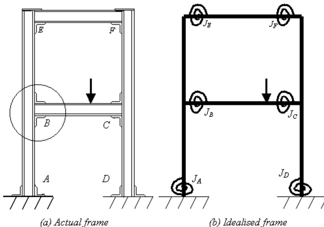
**Fig. 1 Steel frame connections and their modelling**
