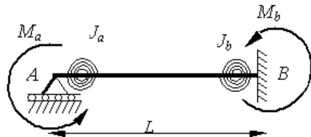
**Fig.7 Beam with far end fixed**
