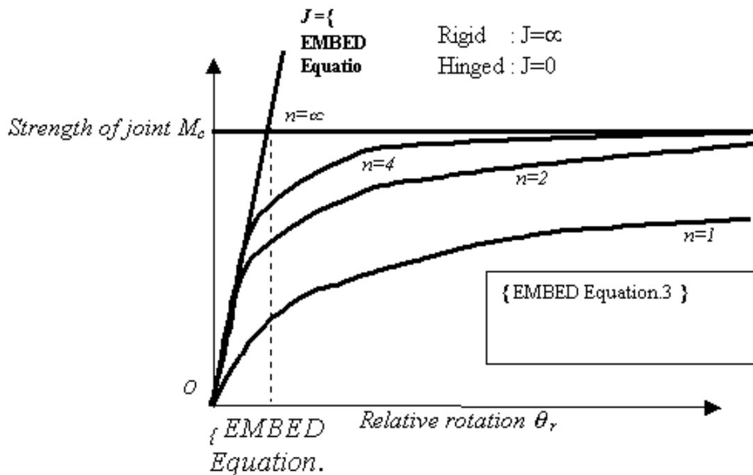
(b) Three parameter model for  $M-\theta_r$  relationship**Fig.5 Connection Stiffness and their representation**
