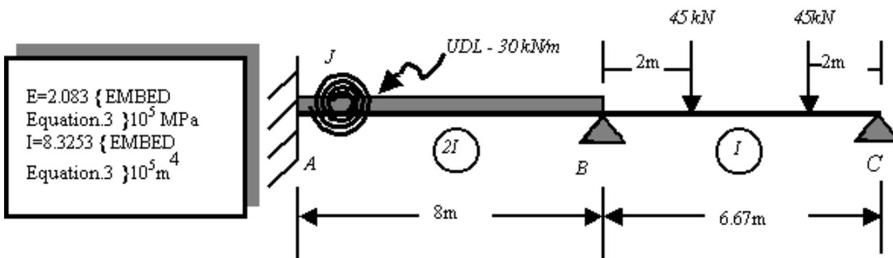
Fig.18 Continuous beam with flexible connection
