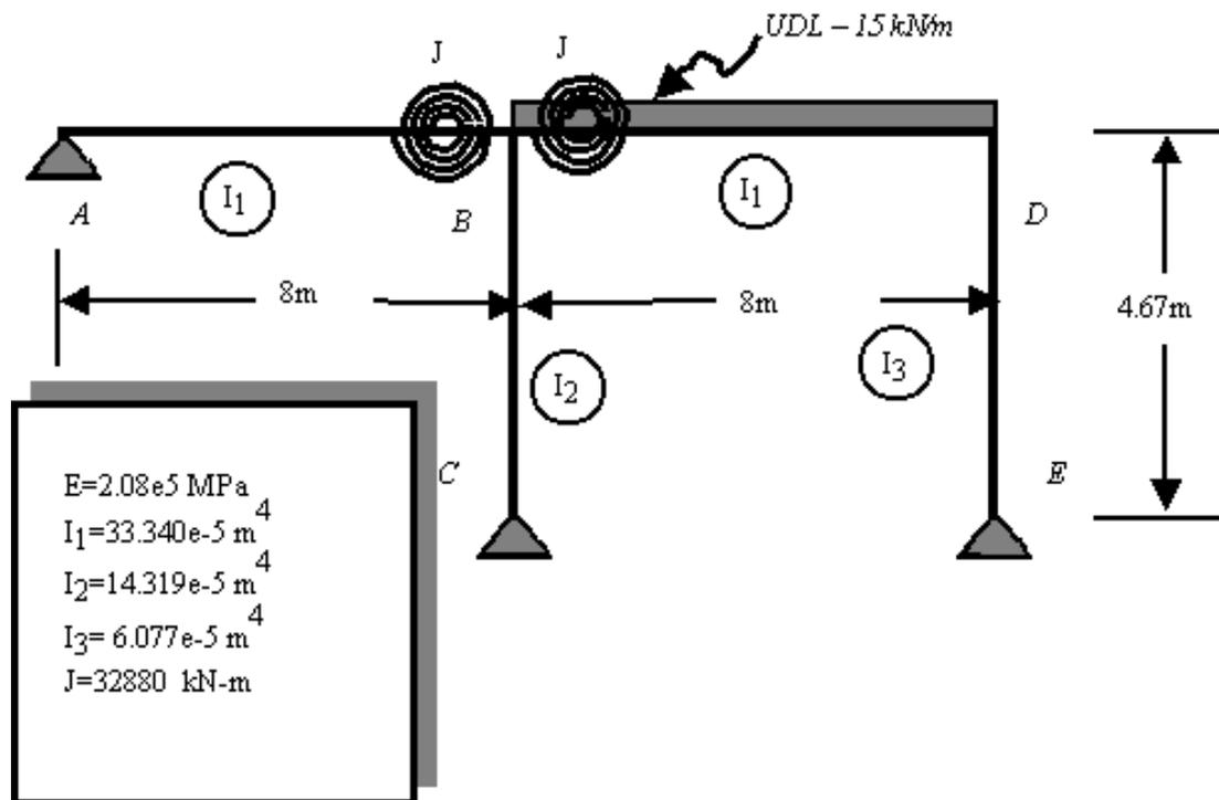
*Fig.20 Single storey steel frame*
