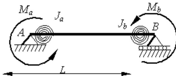
**Fig.6 Beam with connection springs at both ends**
