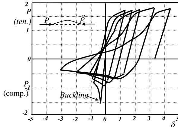
**Fig. 6** *Hysteretic behaviour of a slender brace*
