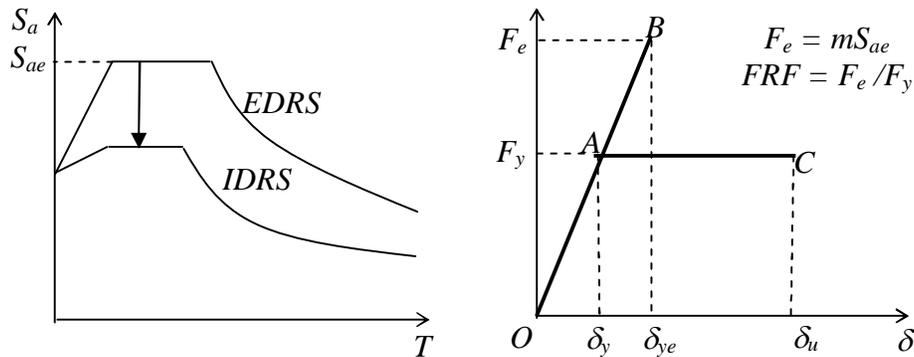
**Fig. 4 Inelastic Design Response Spectrum**
