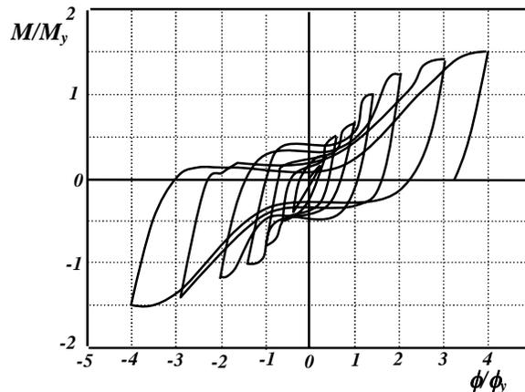
**Fig. 12 Hysteretic behaviour of bolted angle connection**
