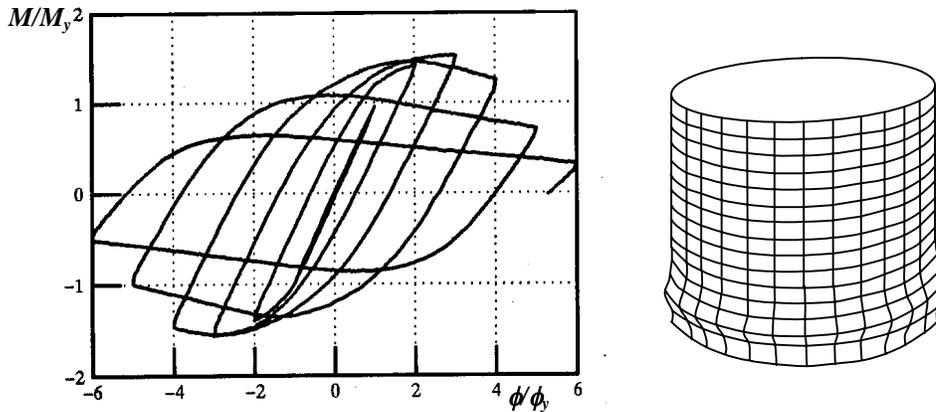
**Fig. 9 Hysteretic behaviour of circular hollow section**
