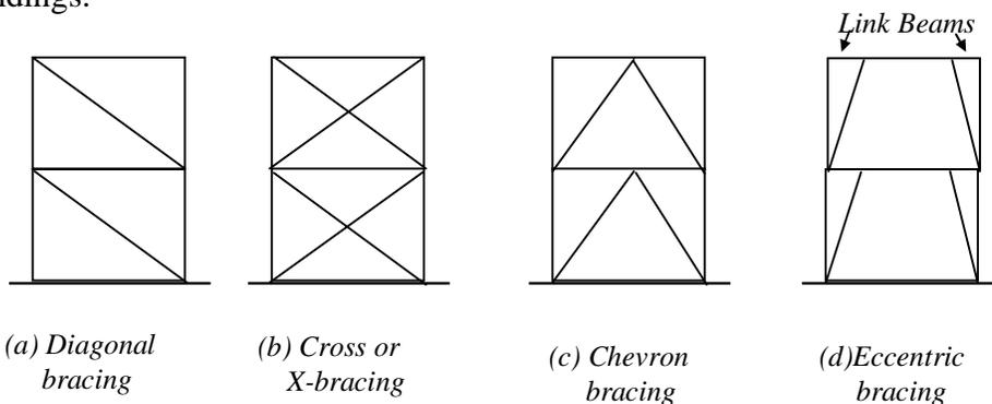
**Fig. 13 Bracing systems in Steel Frames**
