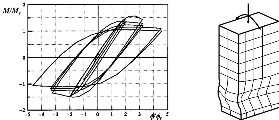
*Fig. 8 Hysteretic behaviour of rectangular hollow section*
