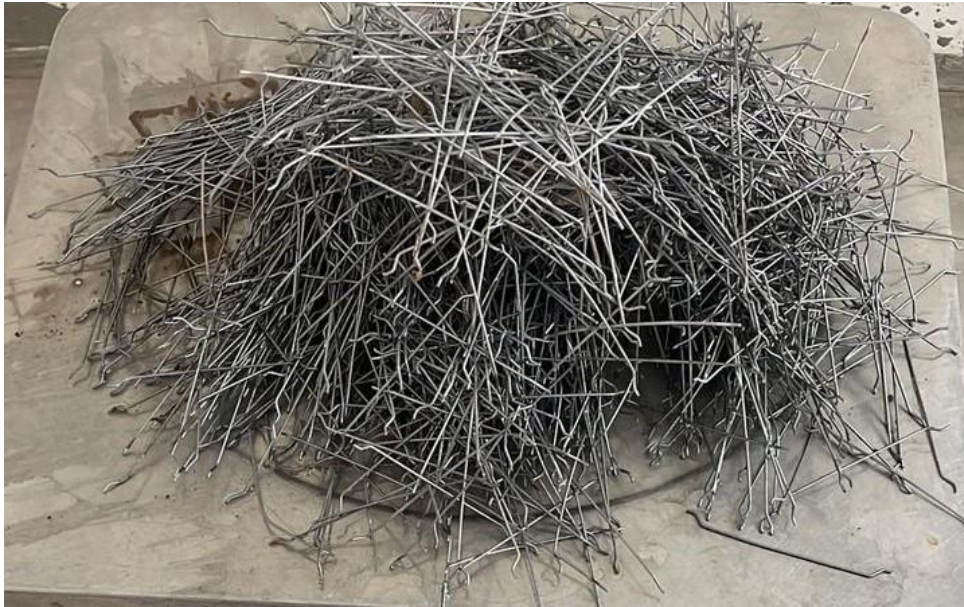
Fig 1: Site Steel Fiber Photos
