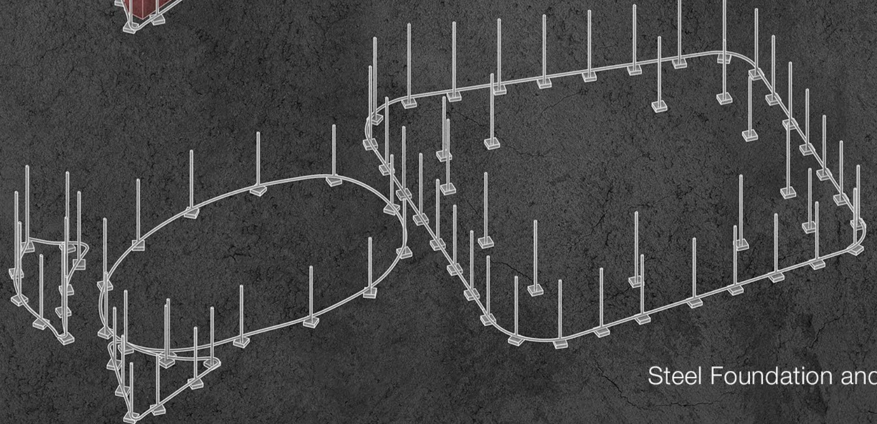
Structural Cores to support the Floor and bridge structure
